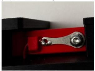
Slide the wire through the hole in the paddle. Then install the M3 hex screws and nuts.
