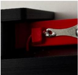
7) On the bottom side place the wire into the slots and connect to the 6-32 screws.
