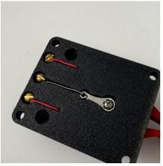
I just strip a portion of the wire and wrap it around the screw, then tighten the nut on the top side.
