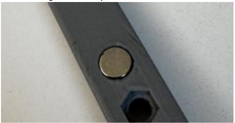
Make sure that the magnets will be in opposing directions from the magnets in the Base. I like to put one of them close to the corresponding magnet in the base which will grab it. Then very carefully use pliers to slide it off of the base magnet, maintaining the correct N-S direction.
